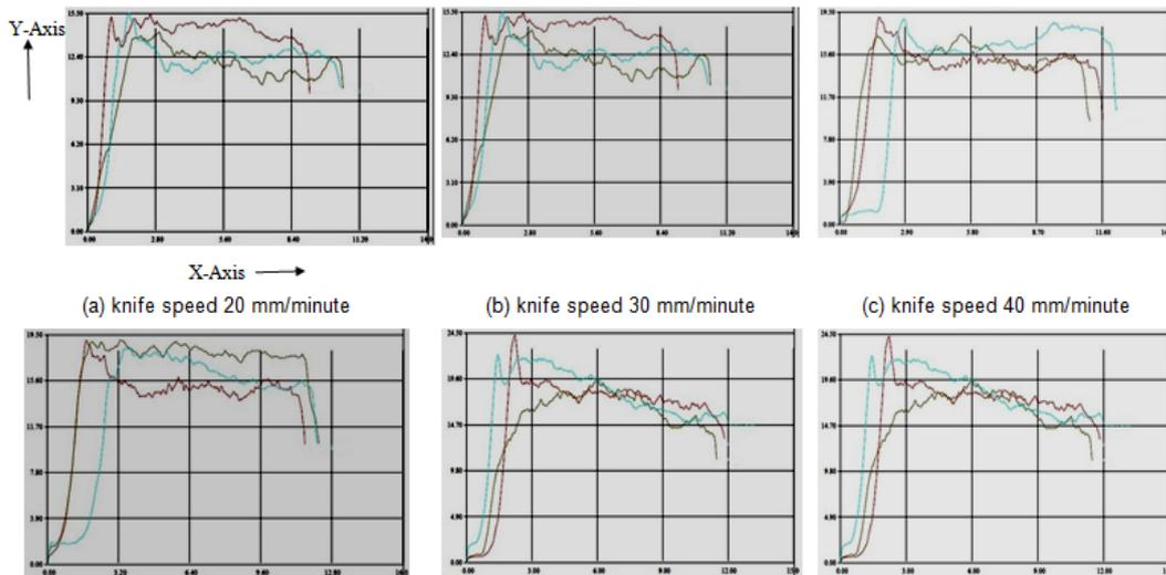
Figure 4. (a-c) and (d-f) Cutting force (Newton, Y-axis) vs. Depth of cut (millimetre, X-axis) for Potato cuboids of contact area (400 and 500 square millimetres respectively), \*Three individual colour lines in graph showing the 3 replicates for each experimental sample
