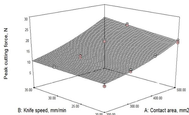
Figure 2. Response surface graph for peak cutting force during transverse cutting of potato as function of contact area (surface area of sample in contact with knife during cutting) and knife speed
