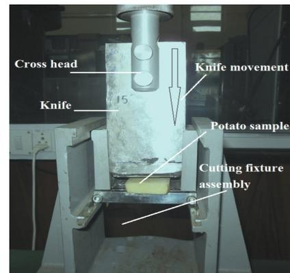
Figure 1. Knife movements in Universal tensile testing machine (UTB-9052, Hi-tech DAK system, load range-500 N) during cutting the potato sample
